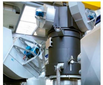
Gas-tight radial fan in two-stage design for transporting hydrogen.
